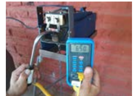
Pyrometer indicating proper blade temperature of 650°C.
